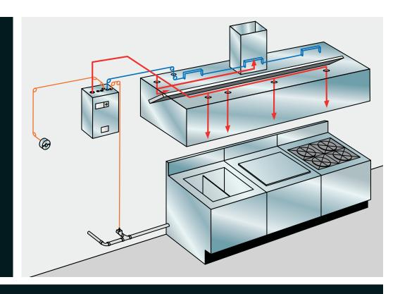
ANSULEX. LIQUID FIRE SUPPRESSANT TWO BASIC DESIGNS WITH PROVEN FUSIBLE-LINK
